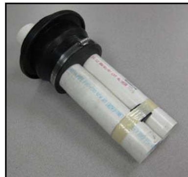
4. Insert the assembled CAST-A-DAPTER through the CAST-A-SEAL® 402 and carefully align the CAST-A-DAPTER with the outside edge of the CAS 402. Tighten clamp to 60 in/lbs using a torque-limiting wrench.
