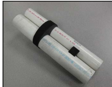
2. Place SPACER PLUG in proper location between the pipes on outside of tank.
