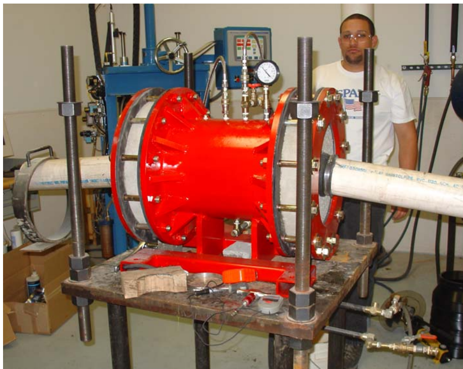
Test Fixture allows simultaneous testing of Infiltration (left) and Exfiltration (right) connector orientations (Angular Deflection Test shown)
