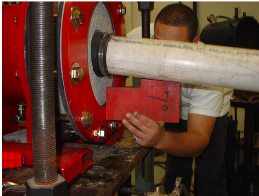
Test Set- Up for Angular Deflection (Exfiltration orientation shown)
