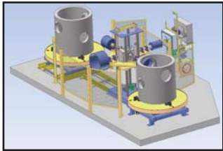
Auto Machine with Two Standard Turntables and Four Rotating Spindles (Bi-Directional Coring)
