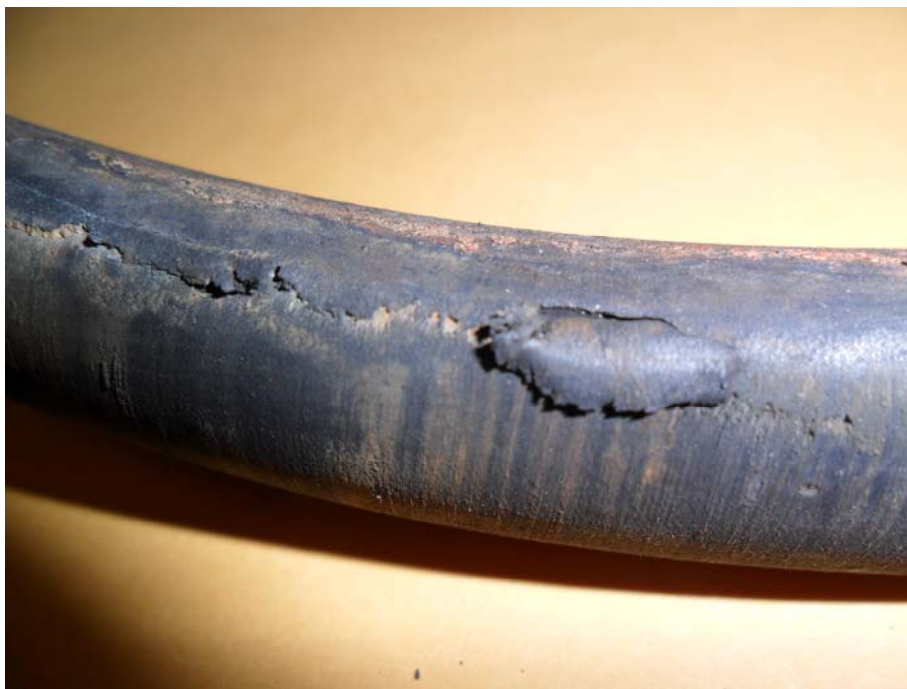
Gasket showing abrasive separation
