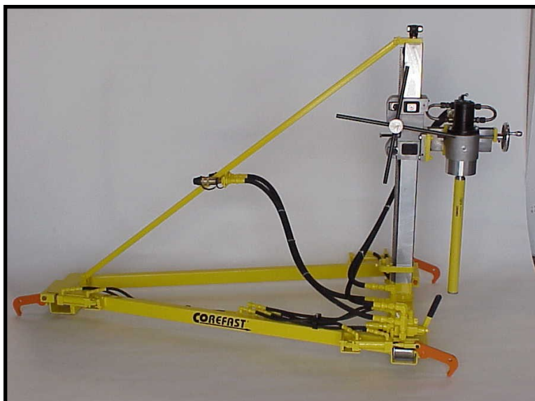
3 Point Integrated Hydraulic Clamping
