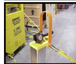
Quick Clamp For Drill Tower Rotation
